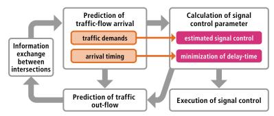
Flowchart for signal control operation
